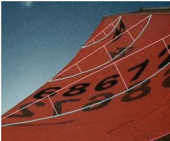
Figure 2: Analysis of sail flying shape.
